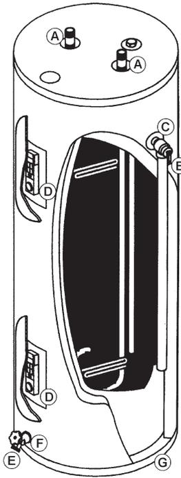
Never use this water heater unless it is completely full of water. To prevent damage to the tank and heating element, the tank must be filled with water. The water must flow from the hot water faucet before turning "ON" power.
