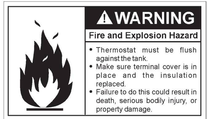
Make sure the thermostat is flush against the tank, the terminal cover is in place, and the insulation is replaced. Failure to do so can result in DEATH, SERIOUS BODILY INJURY, OR PROPERTY DAMAGE.
