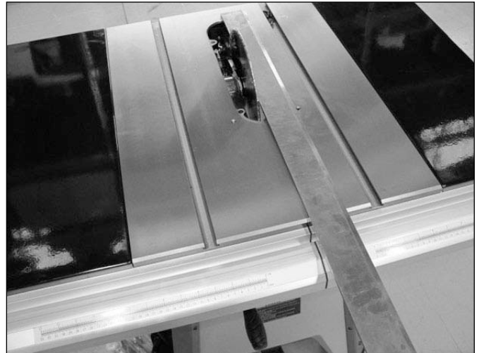
Figure 22 - Use Straight Edge to Align Rail Joint to Blade
